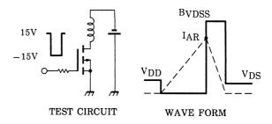
$$\begin{array}{ll} R_G \!=\! 25\Omega \\ V_{DD} \!=\! -50V, \; L \!=\! 10.5 \text{mH} \end{array} \quad E_{AS} \!=\! \frac{1}{2} \cdot L \cdot I^2 \cdot (\frac{B_{VDSS}}{B_{VDSS} \!-\! V_{DD}})$$
