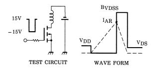
$$\begin{array}{ll} R_G \!=\! 25\Omega \\ V_{DD} \!=\! -50V, \; L \!=\! 12.6mH \end{array} \quad E_{AS} \!=\! \frac{1}{2} \cdot L \cdot I^2 \cdot (\frac{BV_{DSS}}{BV_{DSS} \!-\! V_{DD}}) \end{array}$$
