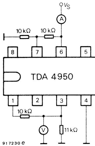
Figure 3 Test circuit 1
