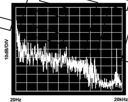
Figure 33. Scope Photo of the 19 kHz FM Subcarrier Frequency
