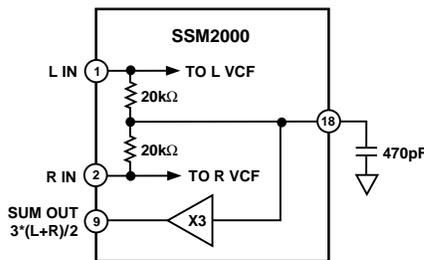
Figure 29. The Internal Circuit for SUM OUT
