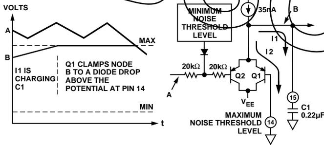
Figure 25a. Condition Where the Actual Noise Threshold Is Above the Maximum Noise Threshold Level Setting (Pin 14)
