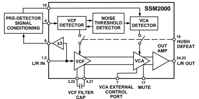
Figure 18. SSM2000 Block Diagram (One Audio Channel Shown)
