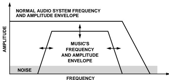
Figure 17. A Frequency-Amplitude Plot of the Audio Envelope
