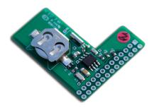
PiFace Real Time Clock means your Raspberry Pi always has the correct time. Furthermore, it's that small you'll hardly notice it's there! You can slip it inside most cases and *under*, most add-on boards!
