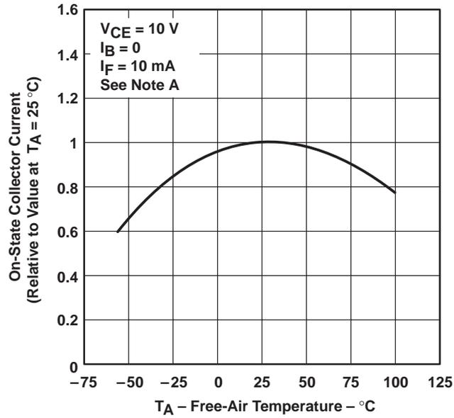
NOTE A. These parameters were measured using pulse techniques,  $t_w = 1\text{ ms}$ , duty cycle  $\leq 2\%$ .
