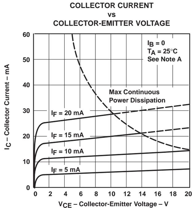
NOTE A. Pulse operation of input diode is required for operation beyond limits shown by dotted lines.
