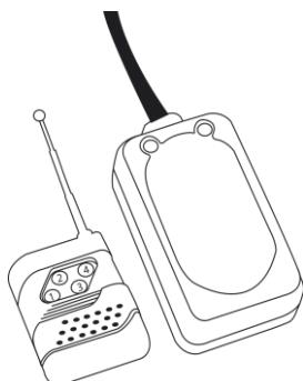
The wireless remote control can control a maximum of 3 devices, in an individual way or all of them at the same time. As it has four button, A, B and C will open the fog spraying for an individual machine, and the D button will do it from three of them at the same time.
