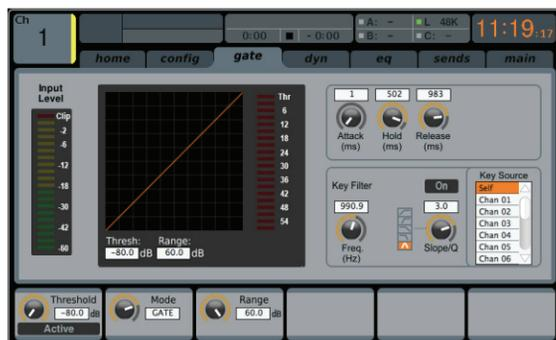
The **gate** tab contains the following parameters, divided among two pages, that can be adjusted using the six push encoders:
