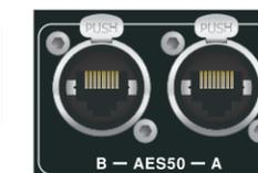
Transmit up to 96 channels in and out via Ethernet cables.
