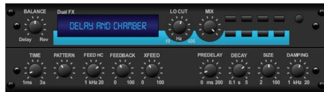
Here we have combined Delay and Chamber reverb, so that a single device can supply a variety of delay settings, plus add just the right amount of reverb to the selected signal. This device only uses one effects slot. *Inspired by the Lexicon PCM 70.*
