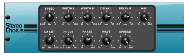
Chorus samples the input, slightly detunes it and mixes it with the original signal to produce a somewhat thicker, shimmering sound. Use it to thicken up background vocals, or to double the sound of brass and woodwind instruments.
