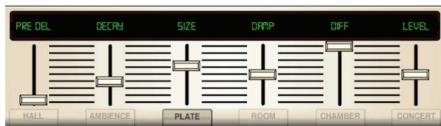
Rich Plate Reverb was originally created by sending a signal through a transducer to create vibrations on a plate of sheet metal which were then picked up as an audio signal. Our algorithm simulates that sound with high initial diffusion and a bright-coloured sound. *Inspired by the Lexicon Plate Reverb.*
