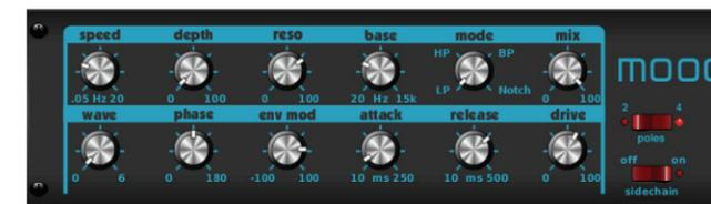
The Mood Filter uses an LFO generator and an auto-envelope generator to control a VCF (voltage-control filter), as well as a side-chain function, where the channel B signal controls the envelope of channel A. When applied to electronic instruments, the Mood Filter can be used to emulate the natural sound of acoustic instruments. *Inspired by the MiniMoog.*
