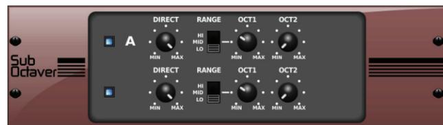
The Octave Effect combines the input signal with a digitally synthesised sound one or two octaves below the original signal. This can be used to thicken up guitar sounds, or to add extra 'punch' to kick drums.
