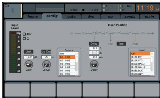
The **config** tab of input channels 1-32 contains the following parameters that can be adjusted using the six push encoders:
