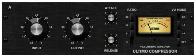
This classic compressor was one of the first audio processors to use Field Effect Transistors. Our digital reincarnation, ULTIMO COMPRESSOR, is based on the early Rev. E model and authentically captures the smooth character of the original class-A output stage and its FET's legendary Fast Attack. *Inspired by Urei 1176LN.*
