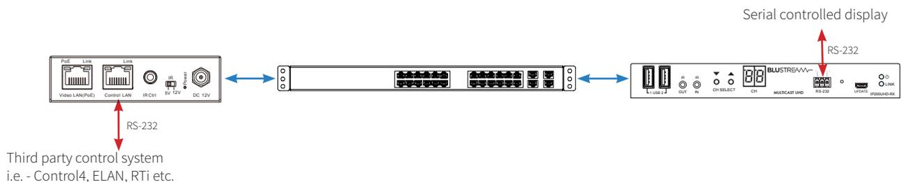
**Please note:** Only one method of RS-232 pass-through can be used at the same time. It is not possible to mix different methods of RS-232 control simultaneously.
