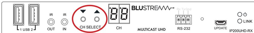
**3) Assign the Receiver ID (IP address)** - once the product is in Local Configuration (LC) mode the display will begin to flash with a lowercase 'r' to indicate the receivers identity is going to be assigned. The identity will also be the IP address that is automatically assigned, so is of utmost importance that an individual ID not equal to another RX unit in the system is assigned:
