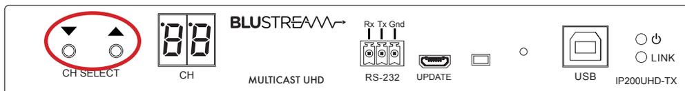
**3) Assign the Transmitter ID (IP address)** - once the product is in Local Configuration (LC) mode the display will begin to flash with a lowercase 't' to indicate the assigning of the transmitters identity. The identity will also be the IP address that is automatically assigned, so is of utmost importance that an individual ID not equal to another TX unit in the system is assigned:
