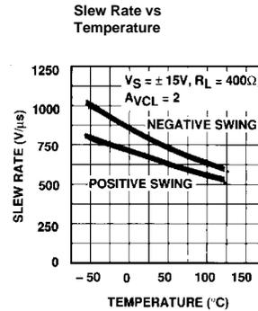
Slew Rate vs Temperature
