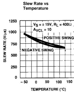
Typical Performance Curves Non-Inverting Gain of One
