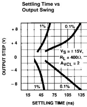
Settling Time vs Output Swing
