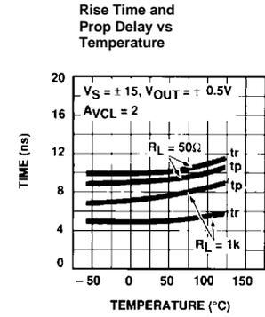
Rise Time and Prop Delay vs Temperature
