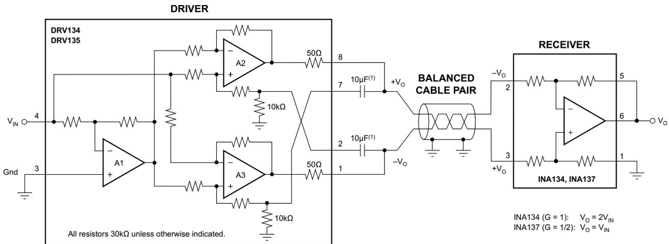
Figure 29. Complete Audio Driver and Receiver Circuit
