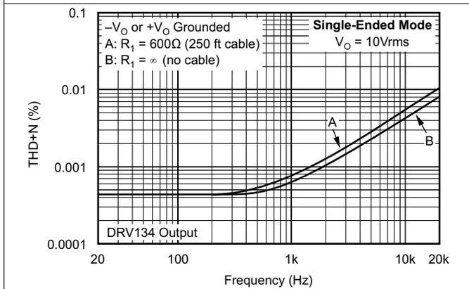
Figure 3. Total Harmonic Distortion + Noise vs Frequency
