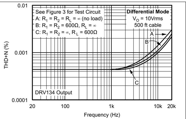
Figure 2. Total Harmonic Distortion + Noise vs Frequency
