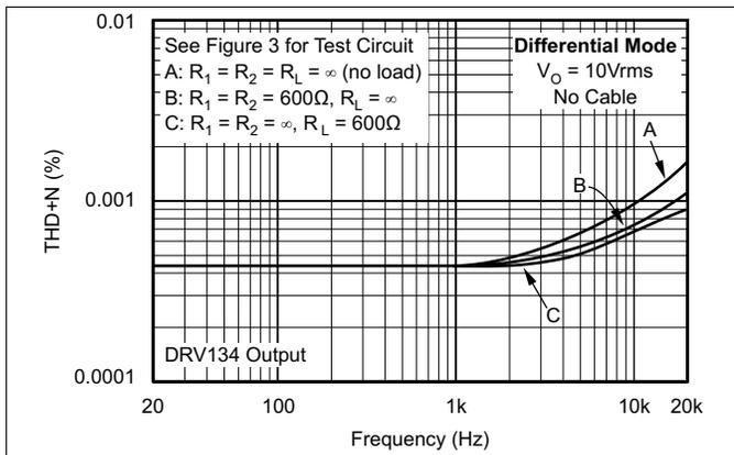
Figure 1. Total Harmonic Distortion + Noise vs Frequency
