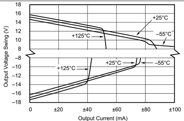
Figure 14. Output Voltage Swing vs Output Current
