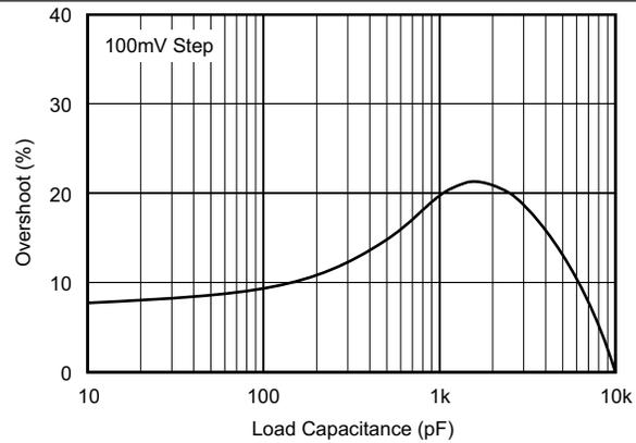
**Figure 23. Small-Signal Step Overshoot vs Load Capacitance**
