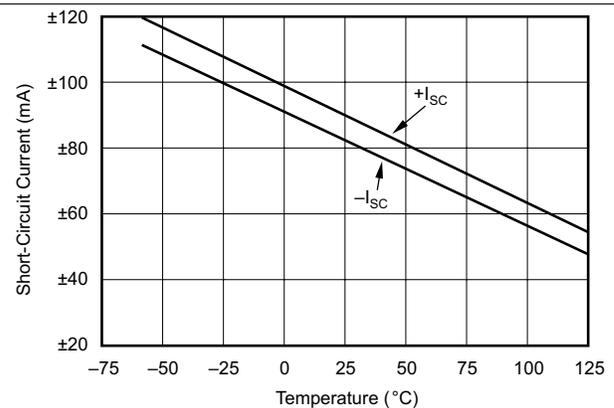
Figure 16. Short-Circuit Current vs Temperature
