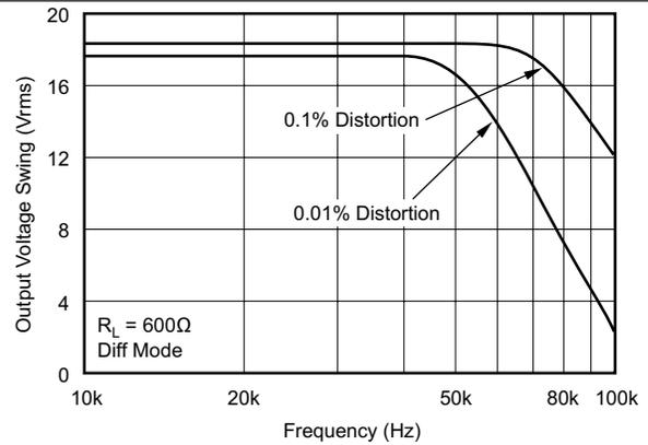
Figure 12. Maximum Output Voltage Swing vs Frequency
