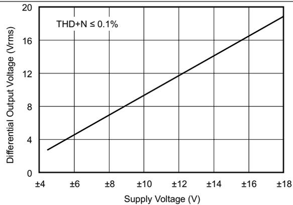
Figure 13. Output Voltage Swing vs Supply Voltage
