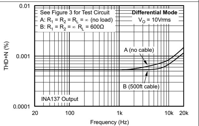
Figure 4. System Total Harmonic Distortion + Noise vs Frequency
