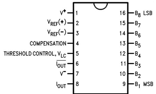
Figure 3. SOIC Package - Top View
