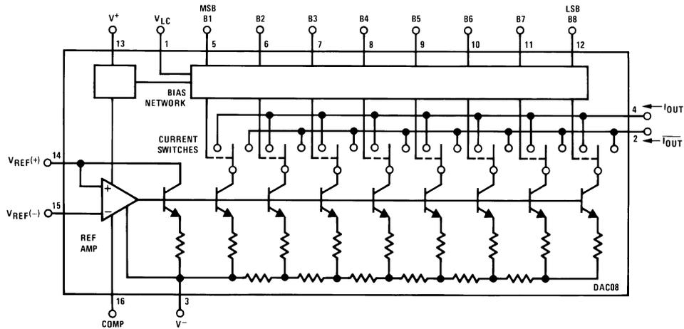
Pin numbers represent the PDIP package. The SOIC package pin numbers differ from that of the PDIP package.
