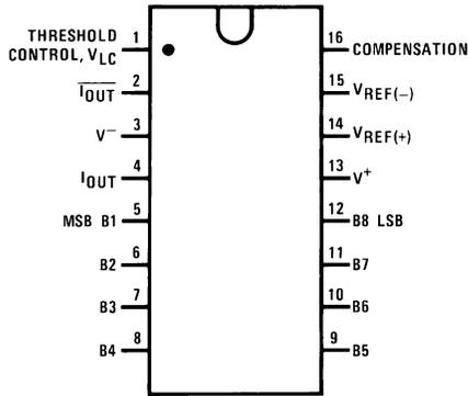
Figure 2. PDIP, CDIP Packages - Top View
