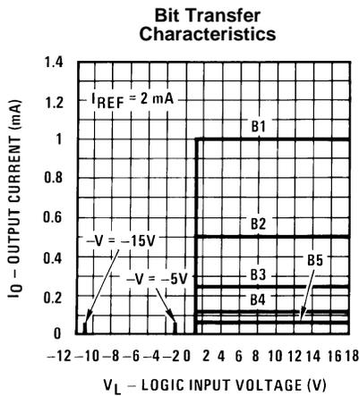
Note. B1–B8 have identical transfer characteristics. Bits are fully switched with less than 1/2 LSB error, at less than ±100 mV from actual threshold. These switching points are guaranteed to lie between 0.8 and 2V over the operating temperature range ( $V_{LC} = 0V$ ).
