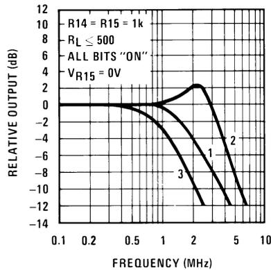
Curve 1:  $C_C=15$  pF,  $V_{IN}=2$  Vp-p centered at 1V.
