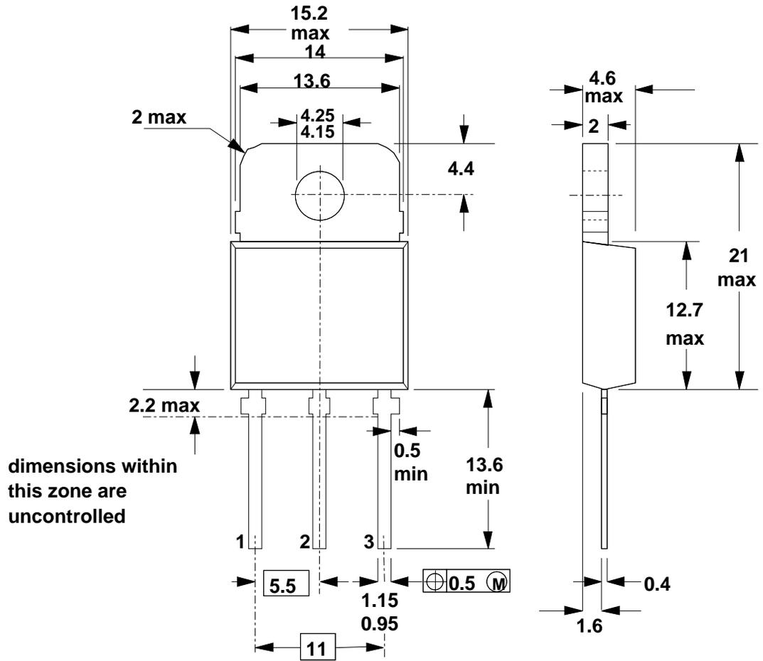
Fig.12. SOT93; pin 2 connected to mounting base.
