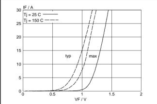
Fig.7. Typical and maximum forward characteristic
