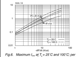
Fig.6. Maximum  $I_{rm}$  at  $T_j = 25^{\circ}C$  and  $100^{\circ}C$ ; per diode.
